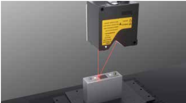
Cover plate warpage measurement
