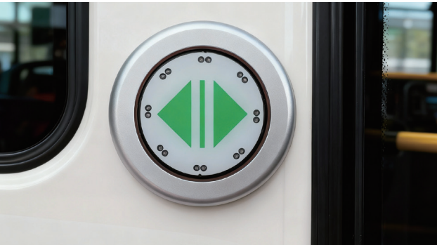
Application of Touch Switches in Coaches
