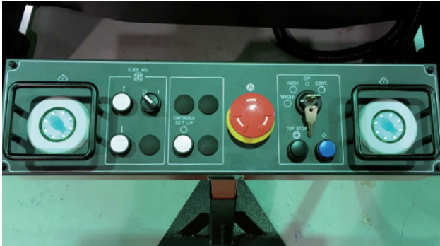
Touch switches in equipment
