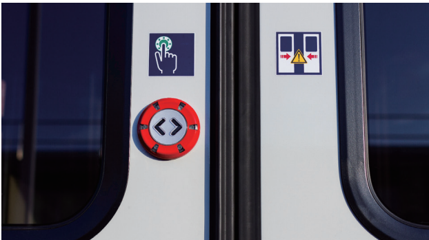
Application of touch switch in high speed rail
