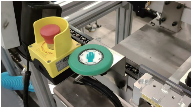
Touch switches in equipment
