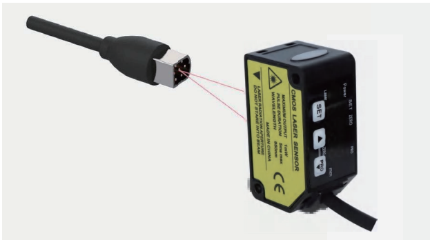
Alignment confirmation of connector pins
